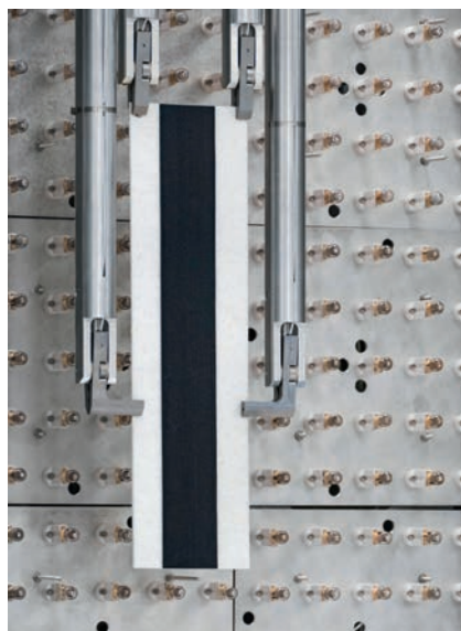
Fig. 1. The high-resolution emitter module (detailed view) enables targeted heating of local amplifications. © KraussMaffei
